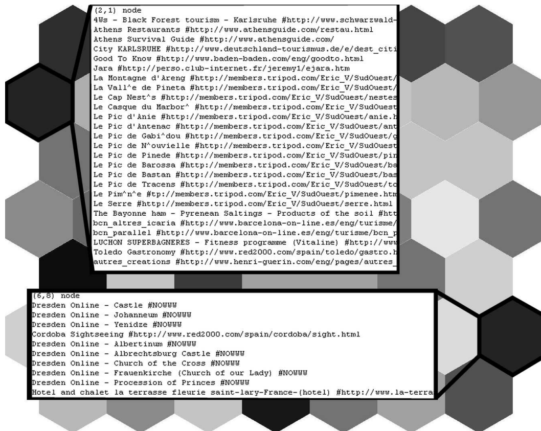
Fig. 8. The document map constructed for the Hypergeo corpus for a 7 \times 7 neural network using the MMWQ-SOM. The document titles as well as their respective URL addresses are listed for each class.
